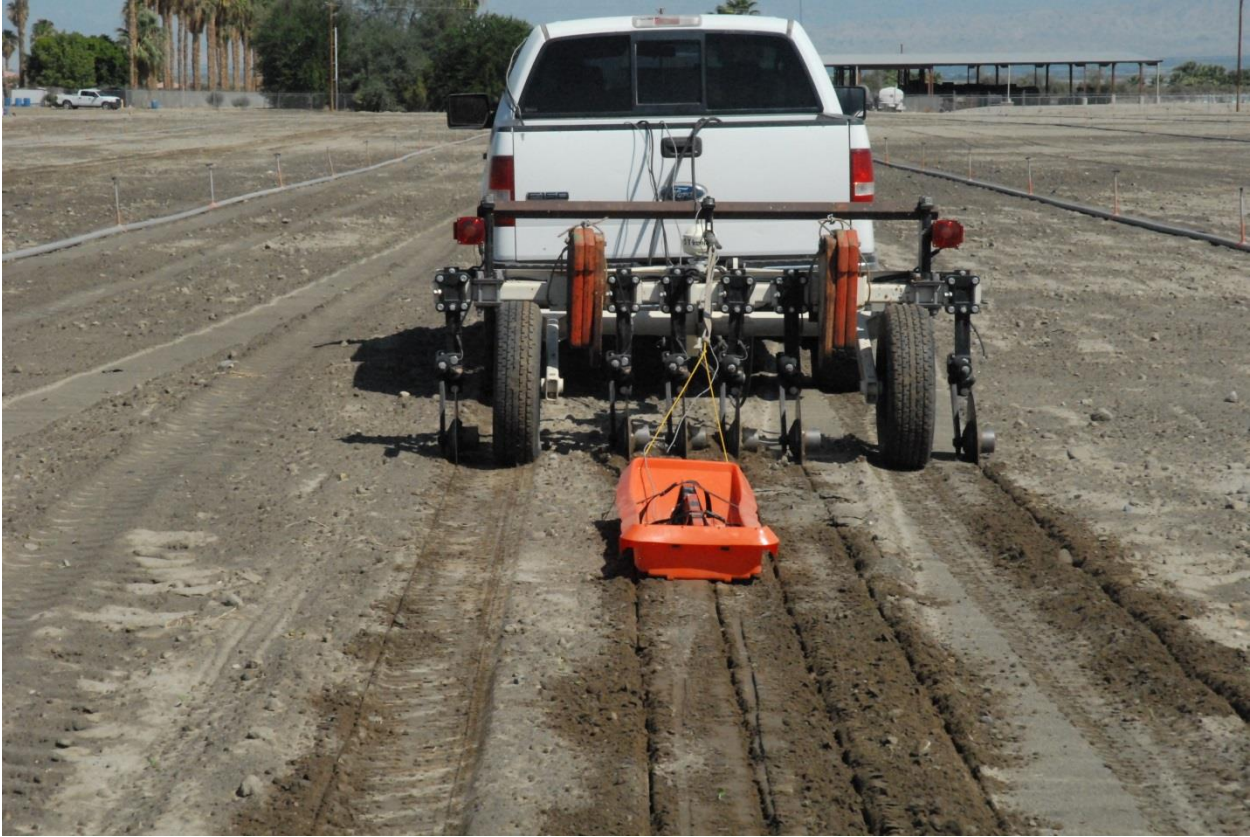
Figure 1. Veris and EM38 survey in the Coachella Valley, Riverside County, CA.
