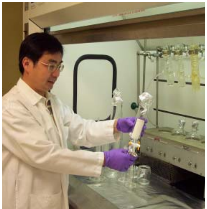
Chemist Charlie Li of the California Department of Toxic Substances Control's Hazardous Materials Laboratory performs soxhlet extraction.
