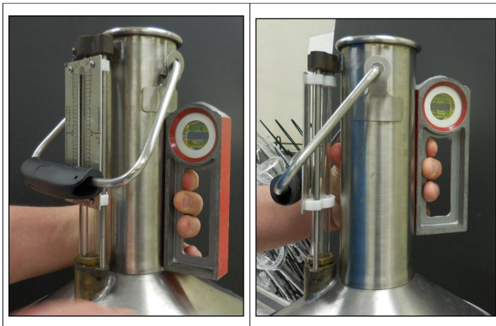
Figure 2 - Level Hand-Held Test Measures on the Neck.
