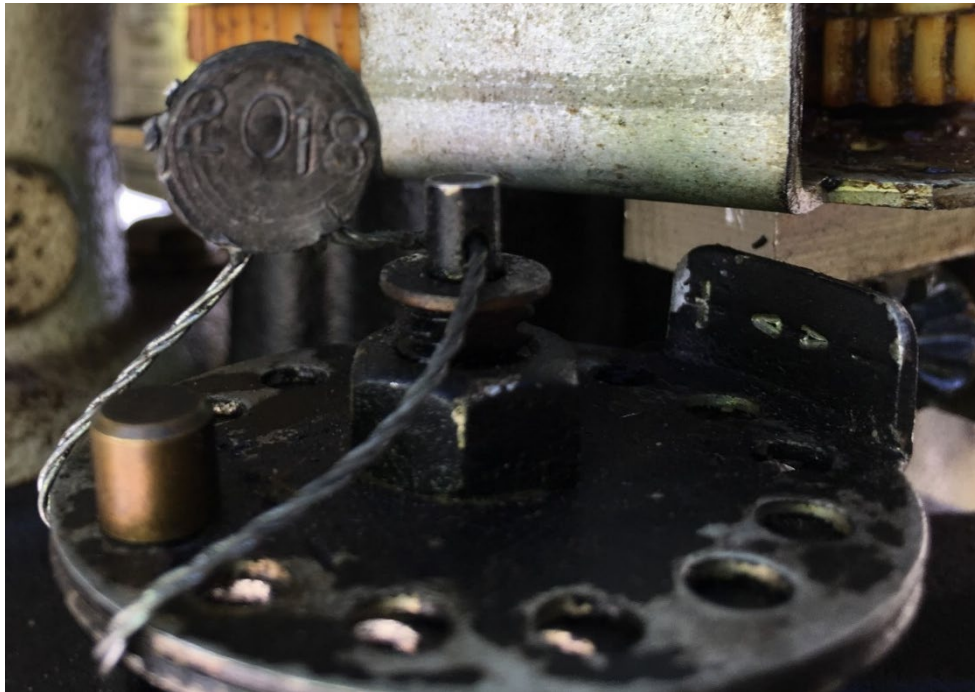
Figure 17 - Example of a Lead & Wire Seal on a Calibration Wheel.
