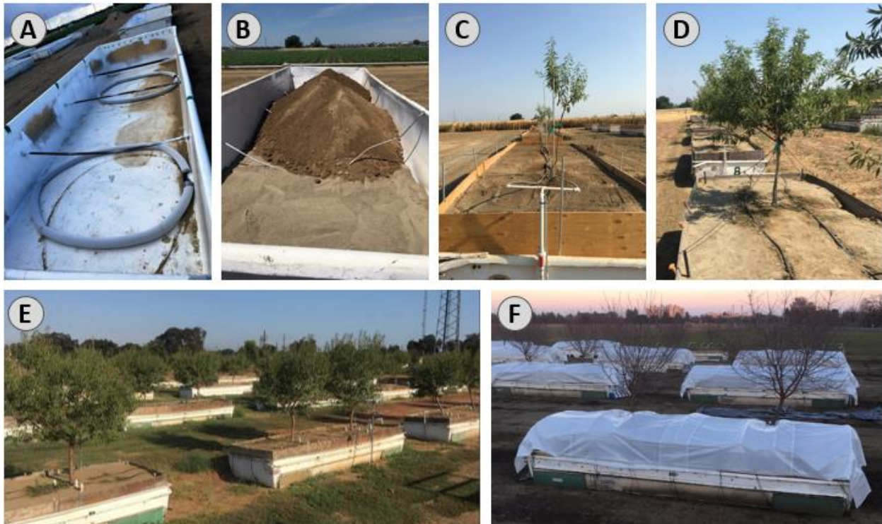
Fig. 1: Construction of the 24 drainage lysimeters. A- Drainage pipe covered with a screen and connected to an outlet in the wall of the tomato truck bin. B- Bin being filled with a layer of coarse sand at the bottom and loamy soil above. C- Young almond trees after transplanting into the bins. D- Trees after having grown in the bins for one year. E-
