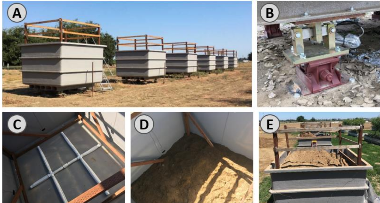
Fig. 2: Setup of the weighing lysimeters. A- Fiberglass bins with railings for safety installed at the experimental site. B- Load cell. C- Drainage system consisting of perforated PVC pipe covered with a screen. D- Bin after adding the first layer of soil. E- Bins after filling with soil and before levelling the soil.
