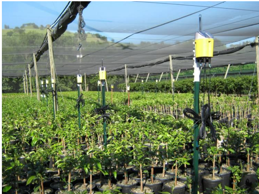
Figure 8. Wireless nodes installed in a container nursery.
