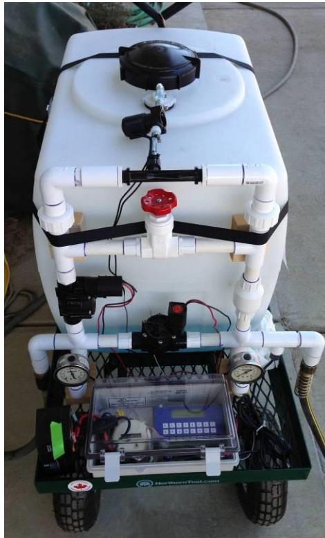
Figure 4. Mobile fertilizer injector with tank, valves, EC sensor, and controller.
