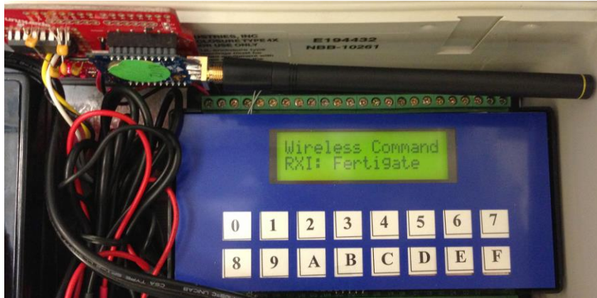
Figure 6. Controller display indicating that a wireless command was received.
