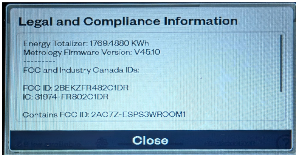
Figure 5. Non-resettable totalizer value and Firmware version example screen
