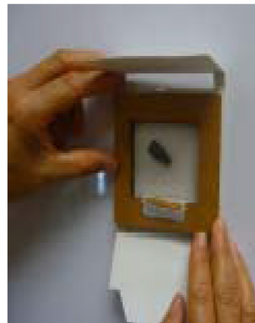
Then remove the cover pad on the adhesive pad and paste the septa. Place carton with food inside cover
