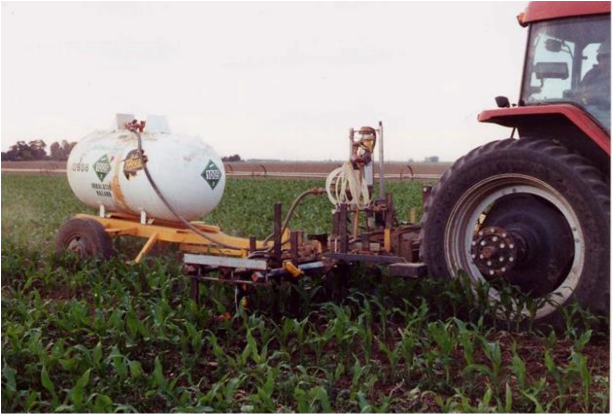
Figure 9. System for precision application of anhydrous ammonia. Electronic rate controller installed in tractor, pulsing valves installed on radial manifold with individual tubes to each knife.
