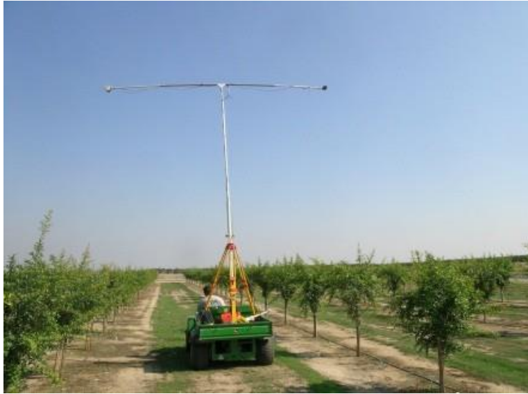
Figure 25. Measurement of canopy cover for pomegranate using TetraCam multispectral camera.
