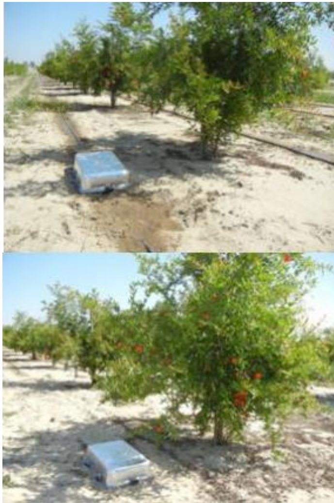
Figure 21. Static chambers used for N 2 O emission measurement and placed above drip tape in surface drip irrigation (top) and subsurface drip irrigation (bottom) systems.
