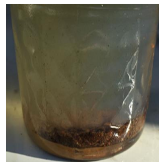
Photos 26 and 27: Diesel fuel contaminated with sediment
