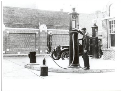
Photos 4 and 5: State officials dispensing gasoline and measuring fuel quantity using a volumetric prover (Seraphin)
