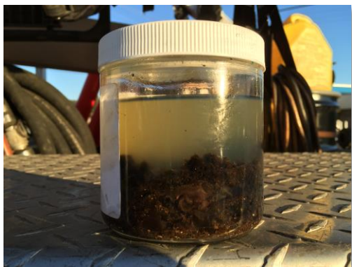
Photo 17: Microbial contamination in No. 2 diesel fuel
