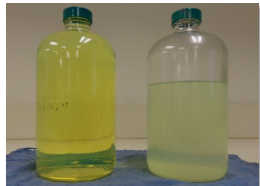
Photo 19: Compliant No. 2 diesel fuel on left. Adulterated No. 2 diesel fuel on right
