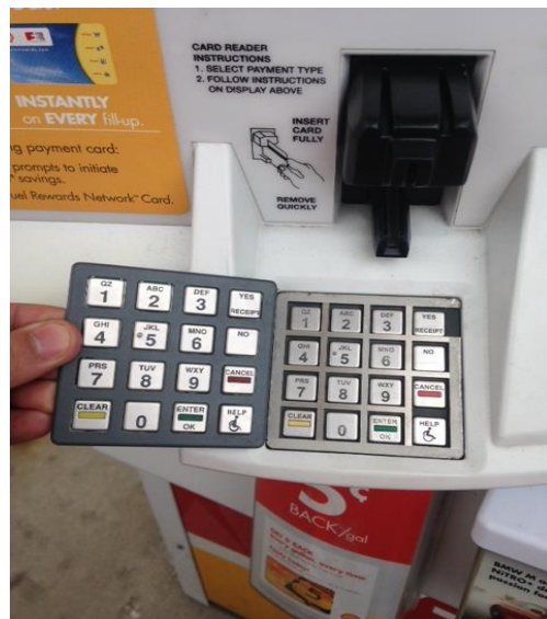
Photo 15: External keypad overlay skimmer
