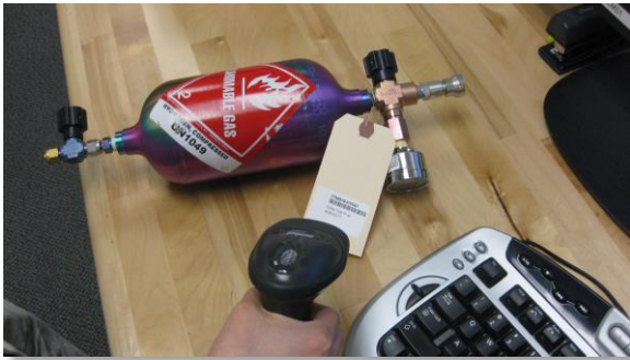
Photo 11: Hydrogen gas container with a LIMS generated bar code label
