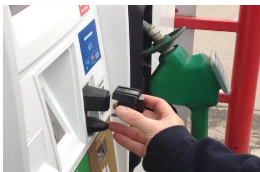
Photo 12: External skimming device being installed on a fuel dispenser
