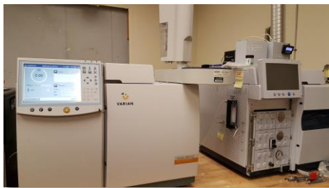
Photos 32 and 33: Gas chromatography instruments used to test various fuel types
