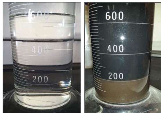
Photo 23: Compliant gasoline on left. Adulterated gasoline on right
